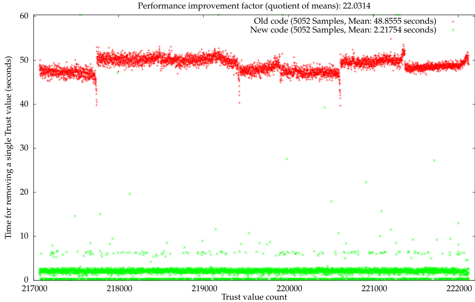
Figure 3.1: Benchmark results of optimized part of incremental Score computation algorithm [53] [54].
